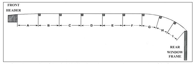
Start from the rear edge of the windshield header and measure to the FRONT edge of the first bow. Then measure from the FRONT edge of the first bow to the FRONT edge of the second bow, etc. Measure all the way to the wood over the rear window. Your car may not have this many rows. Please provide the measurements in "inches" and send this dimension sheet with your order as this information is necessary to make your kit.
