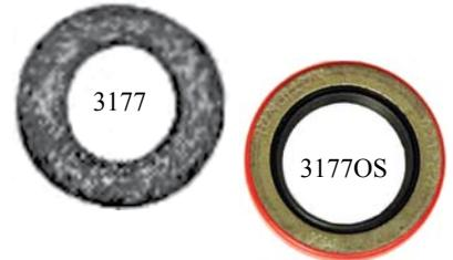
**Lang's Tech Tip:** The area in the timing cover where the seal mounts varies in diameter and occasionally this seal fits loosely in the timing cover. To fix this situation place the seal in a vise between two pieces of wood and squeeze front and back sides together which will increase the outer diameter and improve the fit.
